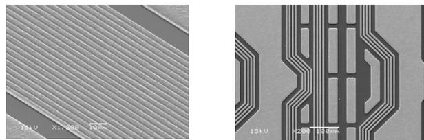
**Figure 4. SEM micrographs of 2/2um LW/LS RDL.**
