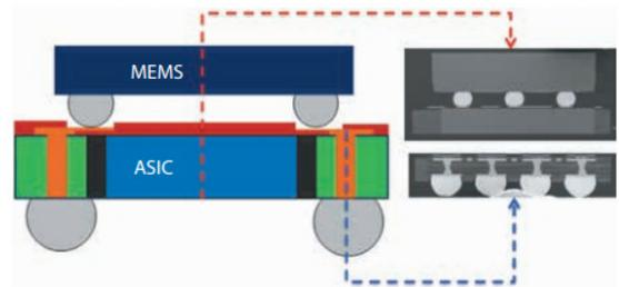
Figure 6. 3D eWLB for MEMS/Sensor Devices[8].
